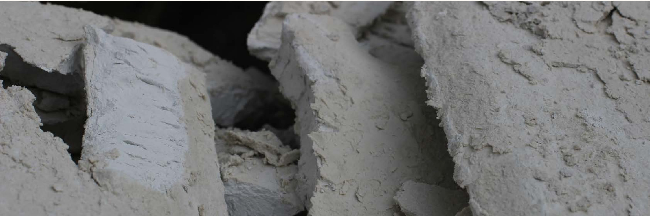
Dry waste following water extraction at our onsite effluent plant - also known as 'paint cake'.
